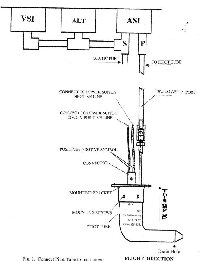
Fig. 1. Connect Pitot Tube to Instrument
